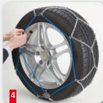
4 Tendere la catena Tighten the chain
